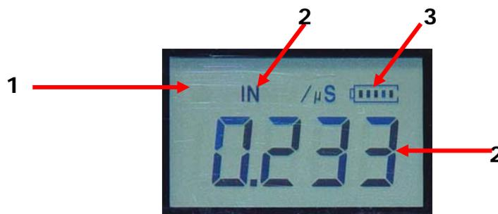
**1, Coupling Indicator:** Indicates the coupling status. While the gauge is taking a measurement, the coupling indicator will be displayed. If it is not, the gauge is having difficulty achieving a stable measurement, and the thickness value displayed will most likely be erroneous.
